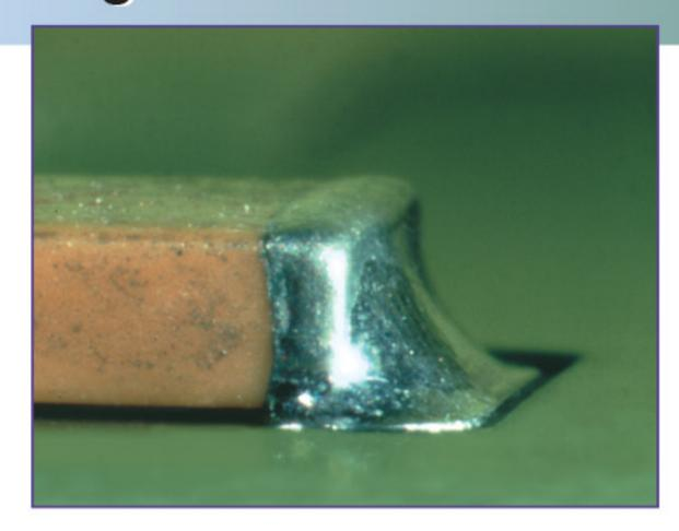
This photo represents a *target* surface mount solder joint for any class of rectangular Chip component.
