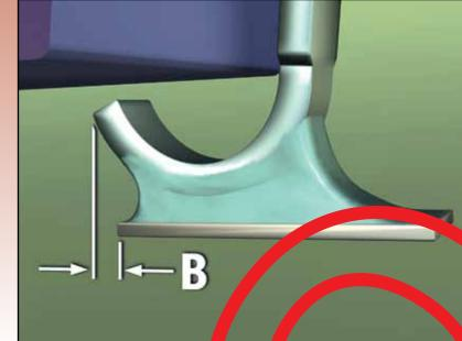
The maximum distance the end, or hip, of the lead may extend over the edge of the land is not specified.
