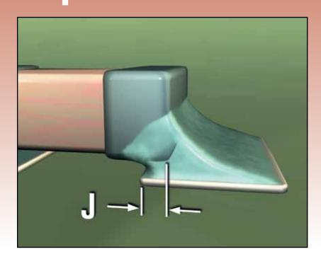
Some amount of overlap between the component termination and the land is required for minimum acceptance.
