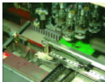
A high speed chip shooter at work.
