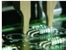
Axial inserter for through-hole components.
