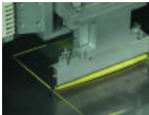
Applying adhesive using the stencil printing method.
