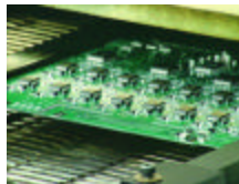
Convection ovens are used to reflow solder paste.
