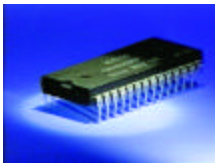
An IC in a Dual-In-Line Package.
