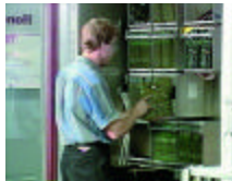
An operator loads assemblies in a thermal chamber for a burn-in reliability test.
