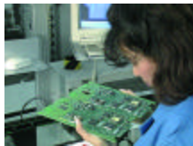
Inspecting a surface mount assembly after component placement.
