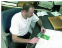
Checking board dimensions during incoming inspection.
