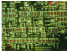
Chip components on the secondary side of the circuit board.
