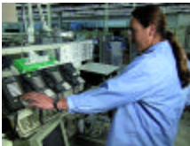
Performing final test on a computerized telephone system.
