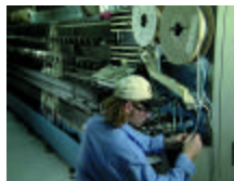
Operator checking newly taped components on a sequencer.
