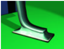
The end result, a surface mounted lead soldered onto a land.
