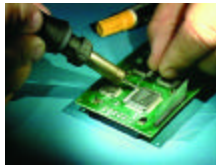
Reworking a bad solder joint.
