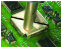
A rework hand tool removes the component.
