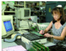
An assembly passes in-circuit test.
