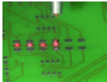
Adhesive dispensing process prior to component placement.
