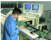
Board inspection after the solder paste printing operation.
