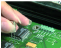
Manual insertion is used for some components.
