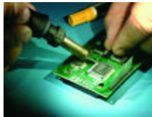
Reworking a bad solder joint.
