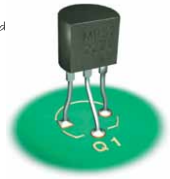
Square land/pad shows pin one orientation
