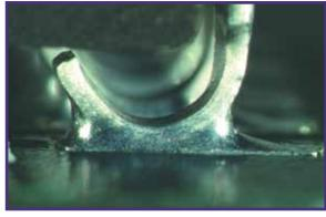
**Notes:** Solder joint drawings are semi-transparent to show relationship between land and lead. Side Overhang, Dimension (A), must not violate minimum electrical clearance. The references below are applicable to the dimensional criteria for J Lead components.
