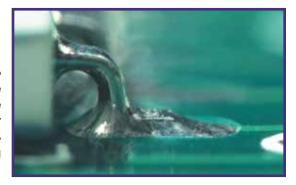
**Notes:** Solder joint drawings are semi-transparent to show relationship between land and lead. Side Overhang, Dimension (A), must not violate minimum electrical clearance. Solder Thickness, or Dimension (G) is not specified for Class 2, only a properly wetted fillet must be evident. Please see Gull Wing, Class 1, for Dim. (G) picture. The references below are applicable to the dimensional criteria for Gull Wing components.
