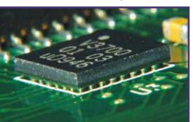
Shows **target** solder connections along the perimeter (visible) row underneath a BGA.
