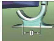
Side Joint Length (D) The length of the solder joint at its narrowest point, must be a **minimum** of 150% the width of the lead (W).
