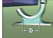
Side Joint Length (D) The length of the solder joint at its narrowest point, must be a **minimum** of 150% the width of the lead (W).
