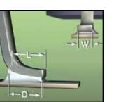
Side Joint Length (D) Short Foot-If foot length (L) is less than 3 (W), then minimum (D) is 100% (L).
