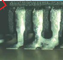
The solder paste had insufficient heat to reflow properly.
