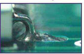
This photo represents an ideal surface mount solder joint for any class of Gull Wing component.
