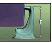
Heel Fillet Height (E) The solder may **not touch** the component body as a maximum fillet height.
