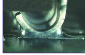
**Notes:** Solder joints are semi-transparent to show relationship between land and lead. Side Overhang, Dimension (A), must not violate minimum electrical clearance. The references below are applicable to the dimensional criteria for J-Lead components.
