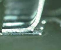
Solder fails to meet minimum heel fillet height. No evidence of properly wetted fillet.
