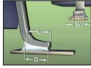
Side Joint Length (D) Short Foot-If foot length (L) is less than 3 (W), then minimum (D) is 100% (L).
