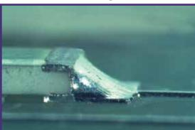
represents an ideal surface mount solder joint for any class of rectangular chip component.
