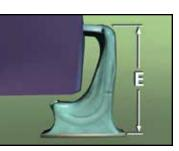
Heel Fillet Height (E) The solder may **not touch** the component body as a maximum fillet height.
