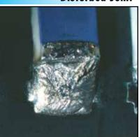
Characterized by uneven surface from movement in the joint while cooling.
