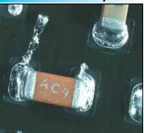
Solder splashes that are not attached, entrapped, encapsulated, that impact form, fit or function, or that violate minimum electrical clearance.
