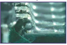
represents an ideal surface mount solder joint for any class of Gull Wing component.
