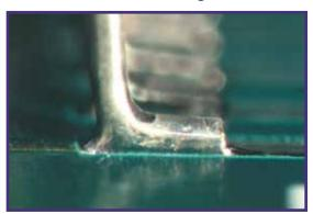
This photo represents an ideal surface mount solder joint for any class of Gull Wing component.
