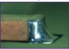
This photo represents an ideal surface mount solder joint for any class of rectangular chip component.
