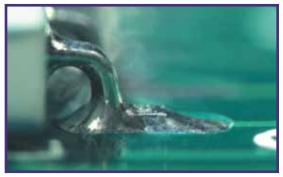
**Notes:** Solder joints are semi-transparent to show relationship between land and lead. Side Overhang, Dimension (A), must not violate minimum electrical clearance for assemblies with small (fine pitch) devices. Solder Thickness, or Dimension (G) is not specified for Class 2, only a properly wetted fillet must be evident. Please see Gull Wing, Class 1, for Dim. (G) picture. The references below are applicable to the dimensional criteria for Gull Wing components.
