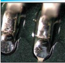
Flux residue from no-clean process on, around, or bridging between noncommon lands, component leads and conductors. Residue does not inhibit visual inspection. Flux residue does not prevent access to test points of the assembly.
