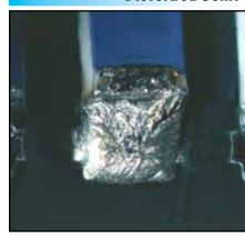
Characterized by uneven surface from movement in the joint while cooling.
