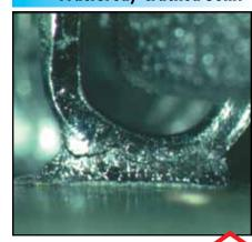
Fractured or cracked solder joint.
