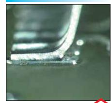
Solder fails to meet minimum heel fillet height. No evidence of properly wetted fillet.
