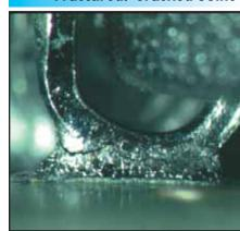
Fractured or cracked solder joint.
