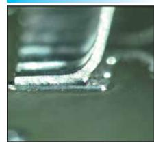
Solder fails to meet minimum heel fillet height. No evidence of properly wetted fillet.
