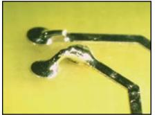
Solder has bridged to adjacent noncommon conductor.
