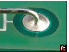
Surface of lead free solder joints may be grainy or dull.
