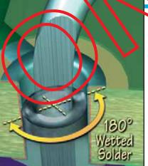
Barrel - Wetting of Lead & Barrel
