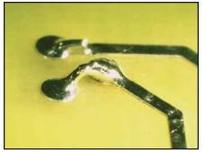
Solder has bridged to adjacent noncommon conductor.
