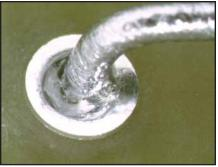
Minimum acceptable condition for vertical fill of solder on Class 1 assemblies is not specified. Less than 100% solder fill may not be acceptable in some applications, e.g., thermal shock.
