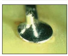
Solder (secondary) side exhibits 360° of good wetting, and coating is not visible within the connection on solder (secondary) side.
