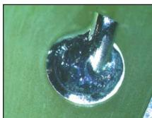
Defect Class 1, 2, 3 Cold solder joint: lumpy and poorly wetted to land and lead.
